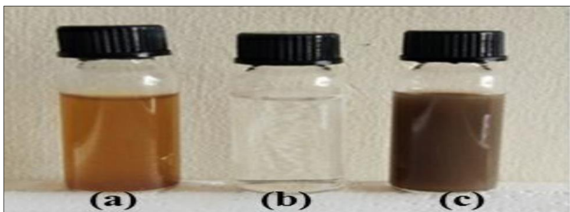
Figure 2 (a) leaf extract (b) AgNO 3 solution (c) Ag NPs
